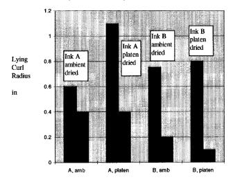
Figure 7. The use of checkerboard printing in minimizing steady state curl. The higher value refers to no checkerboard printing, the lower value to checkerboard printing.
