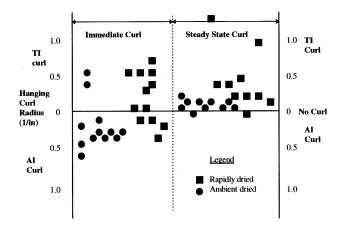
Figure 5. Curl development as function of drying rate.
